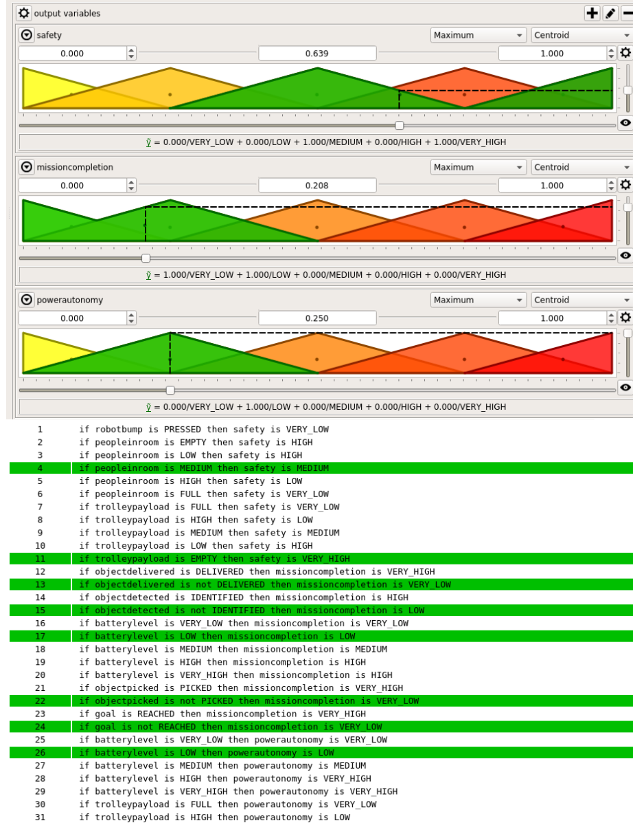
Fig. 3: (Top) Evaluation of high-level perceptions using fuzzy logic: (safety, missioncompletion and powerautonomy; and (Bottom) Rules set for determining the current high-level perceptions
